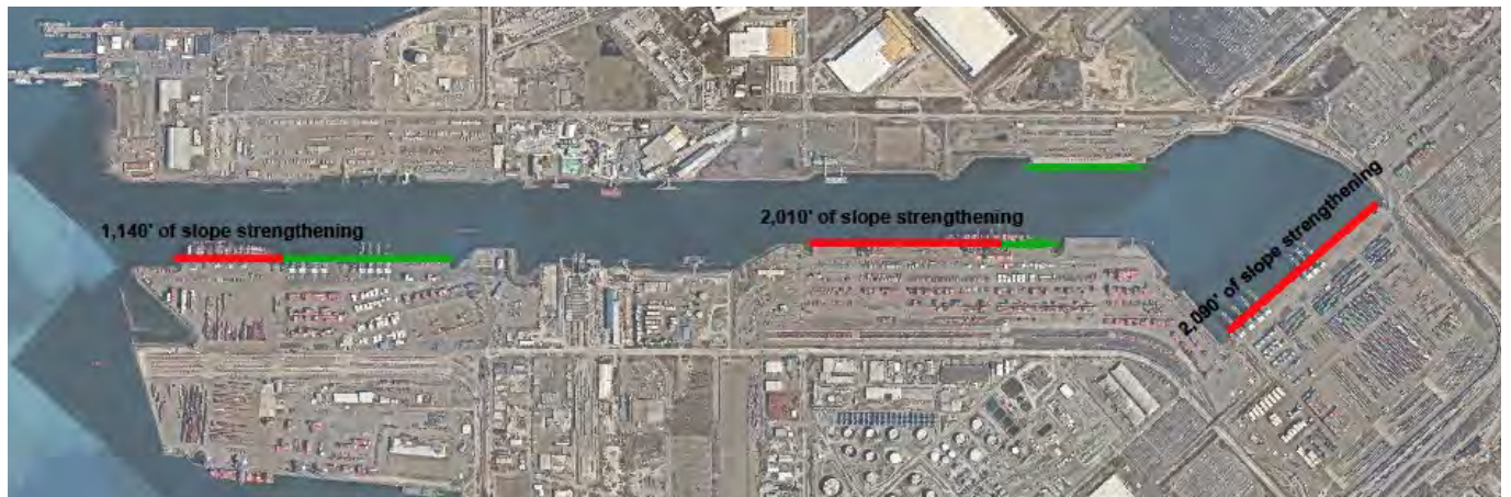
Figure 5. Anticipated Slope Strengthening by Facility for Depth Below -54 MLLW.
